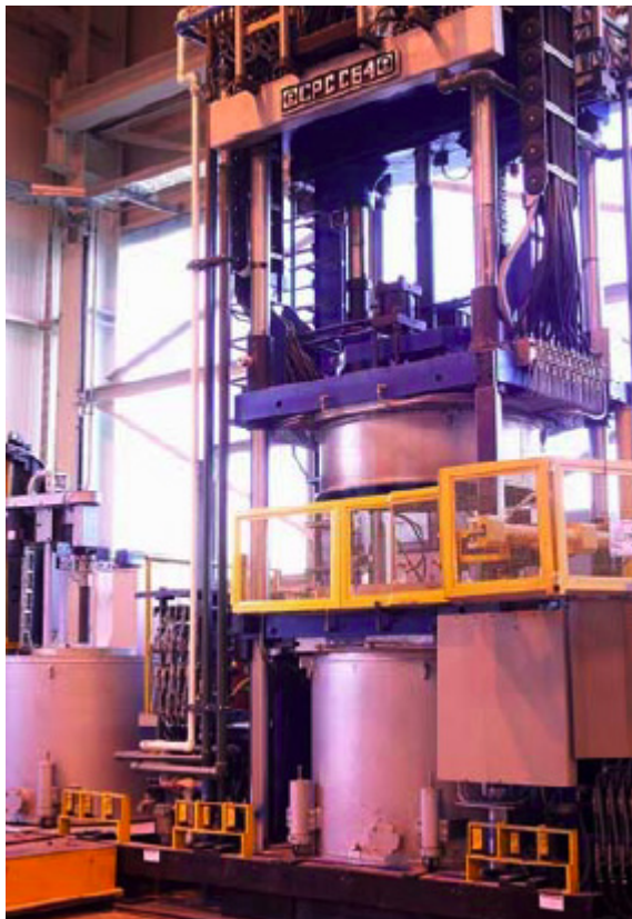
Picture: Counter-pressure permanent mold casting facility at ThyssenKrupp Fahrzeugguss GmbH in Hildesheim, Germany.
